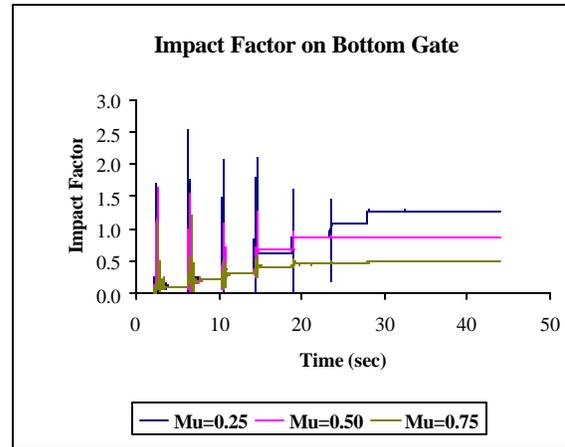
Figure 7. Effect of coefficient of friction on bottom gate impact factor
