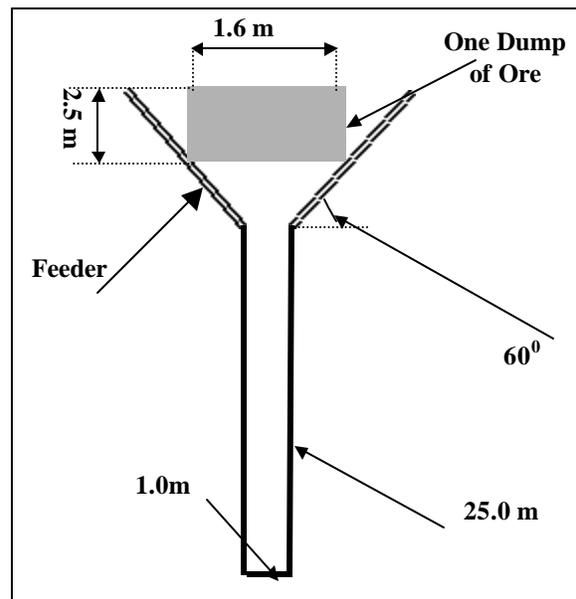
Fig. 5. Ore pass configuration (not to scale)
