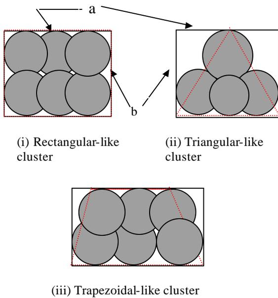
Fig. 4. Three different shapes of ore-clusters
